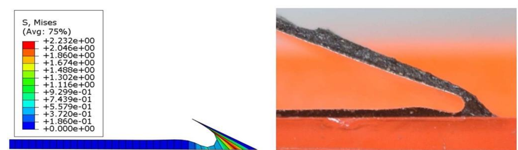
Figure 6 – Simulation vs. experimental deformation comparison image.
