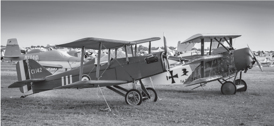
Figure 1.3. Aircraft of bonded wooden construction used during World War I.
