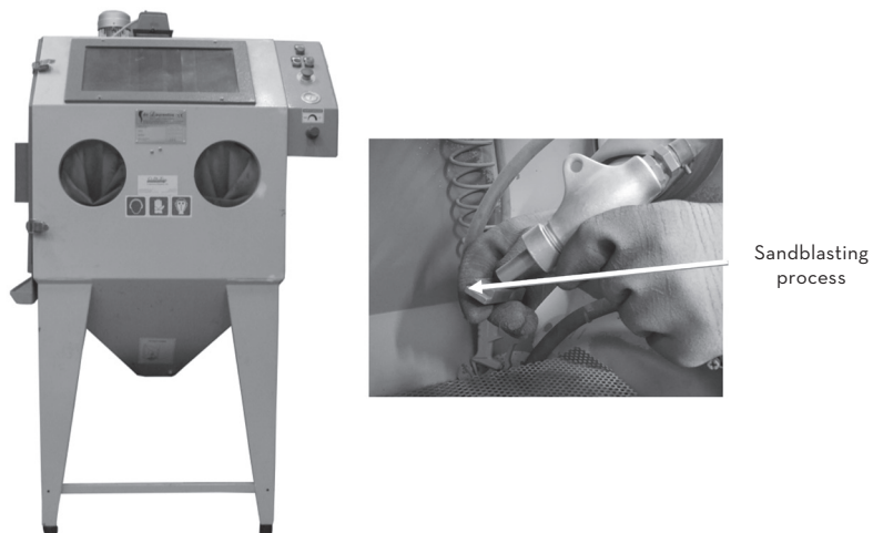
Figure 3.4. Sandblasting process of metallic substrates.
