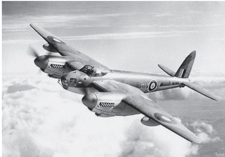
Figure 1.4. The deHavilland Mosquito, a World War II high performance aircraft built of wood and bonded with structural adhesives.
