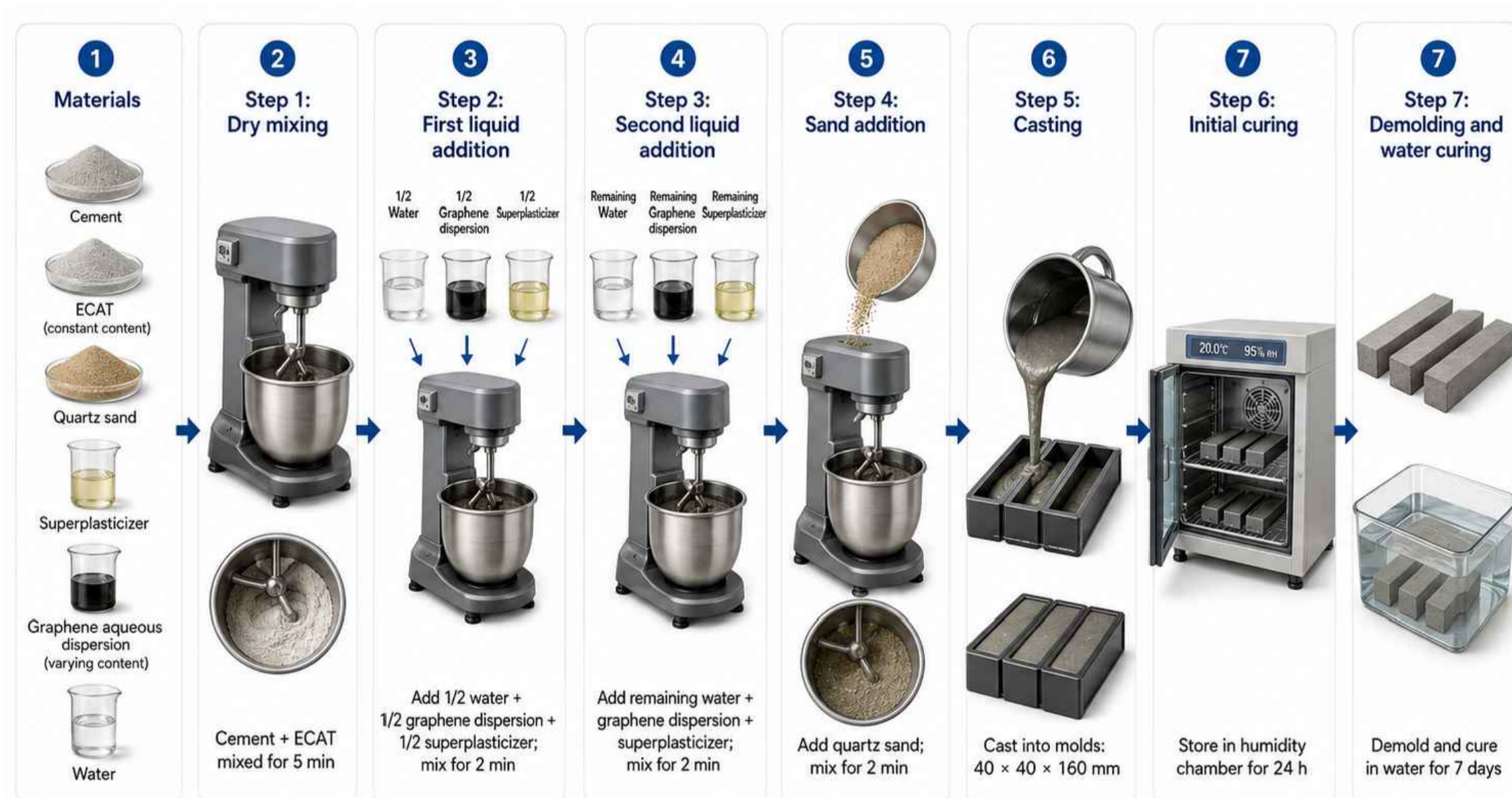
Fig. 3. Scheme of cementitious sample preparation
